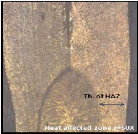
Fig. 15 Microstructure of weld zone for sample 4
