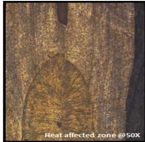
Fig. 16 Microstructure of weld zone for sample 5
