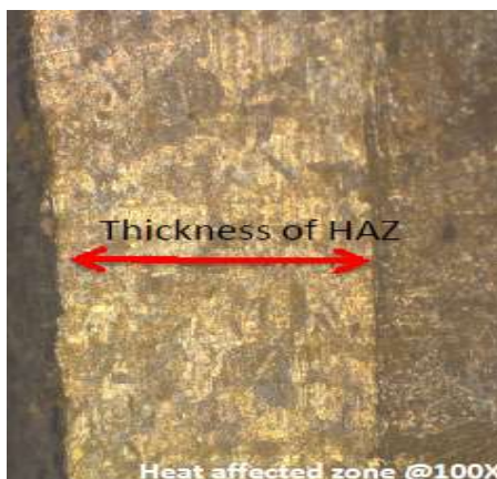
Fig. 13 Microstructure of weld zone for sample 2
