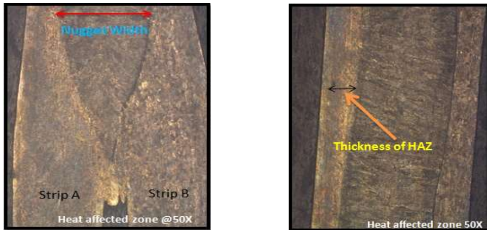
Fig. 23 and Fig. 24 Microstructure for weld zone and heat affected zone for sample 9 At 50X magnification
