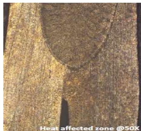
Fig. 14 Microstructure of weld zone for sample 3
