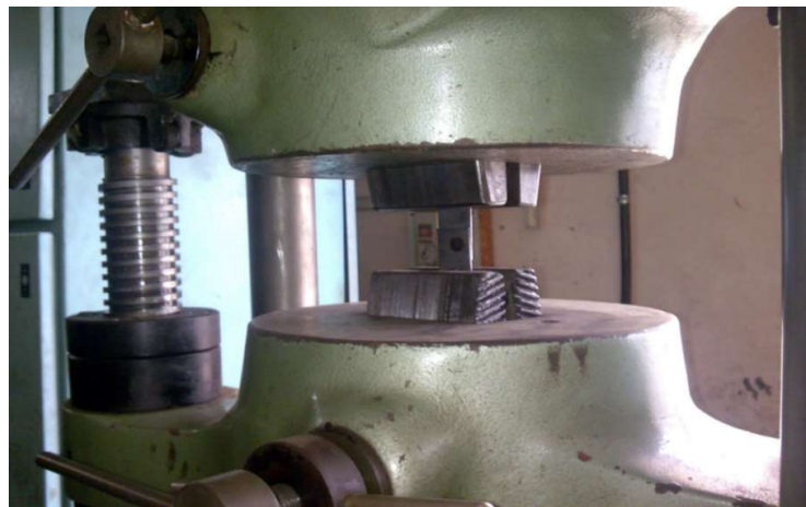
Fig. 7 Clamping of specimen on UTM
