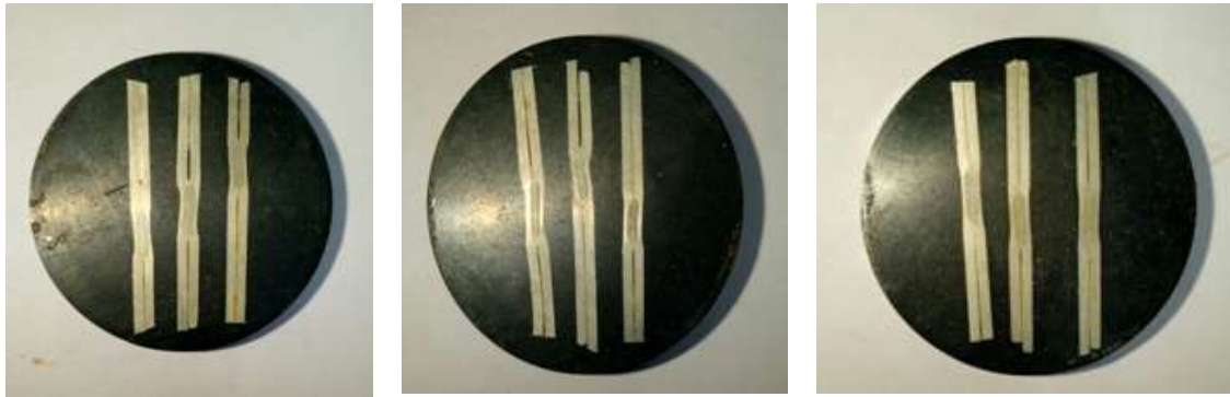
Fig. 8 Mould of a sample after polishing and moulding process
