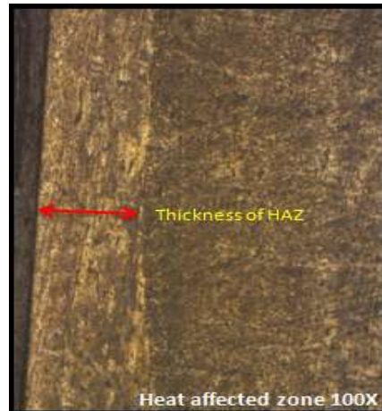
Fig. 17 and fig. 18 Microstructure for weld zone and HAZ for sample 6 At 50X and 100 X magnification
